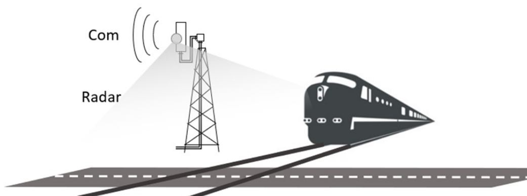
Figure 7. RADAR sensing of a Railroad Crossing to provide an early warning to the train driver.
