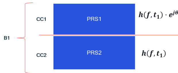
Figure 16: PRS frequency stitching, where CC means component carrier and \theta random phase offset between both CCs from [32],[33]
