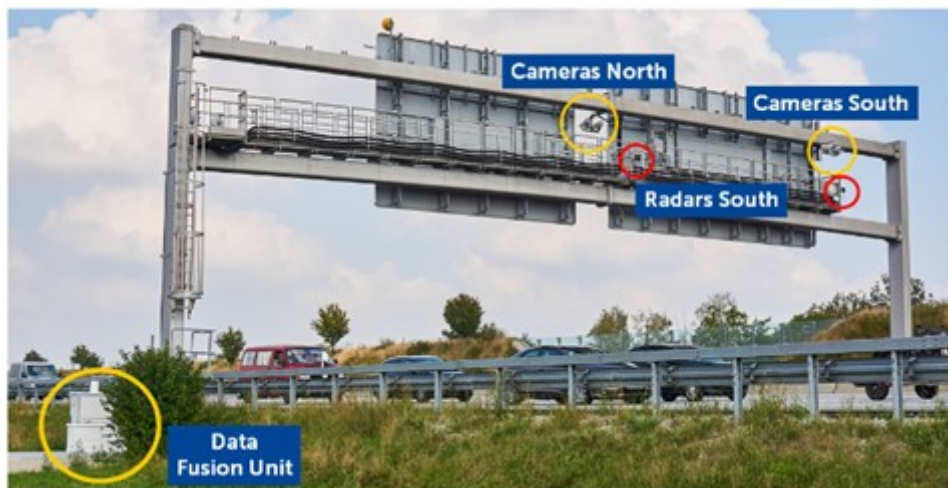
Figure 2.8: An example of the measurement points installed on the A9 highway near Munich, Germany. In addition to the visible radars in this picture (indicated by the red circles), two further radars directed towards the north are installed on the other side of the gantry and cannot be seen from this perspective [33]
