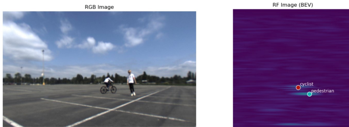
Figure 3.3: Cross-modal sensing with camera imaging and static FMCW radar, scenario A [11].
